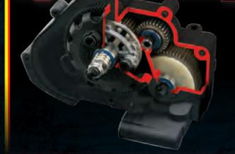
Torque-Control® Slipper Clutch
